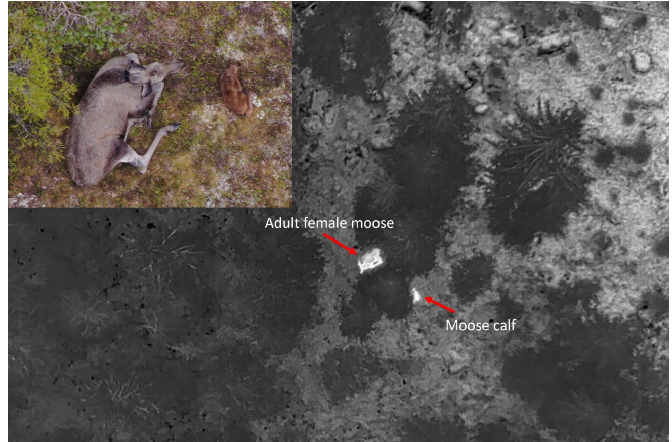
Fig. 5: Example of a thermal image taken by the DJI Matrice 300 RTK Combo drone equipped with a dual camera that recorded both thermal infrared TIR and color RGB (DJI ZenMuse H20T). The small image shows an image taken with the zoom camera (500 mm) from a different moose cow and calf. Pictures: Thomas Vogler.
